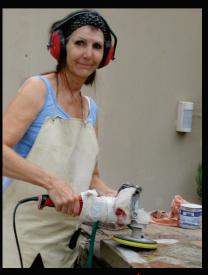
Rock slices were cut using an angle grinder (above left), then embedded into cement (over middle) then ground smooth and polished (above right)
