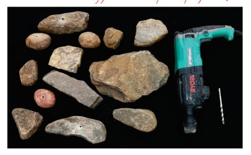
Above-flat rocks or ones that are not too thick for a drill bit to get through. If they are, one drills as far as possible from one side, then turn it over and aligns the bit so the two holes meet up. Either a drill press or a hand drill works well but ALWAYS use water else the bit will burn out.
